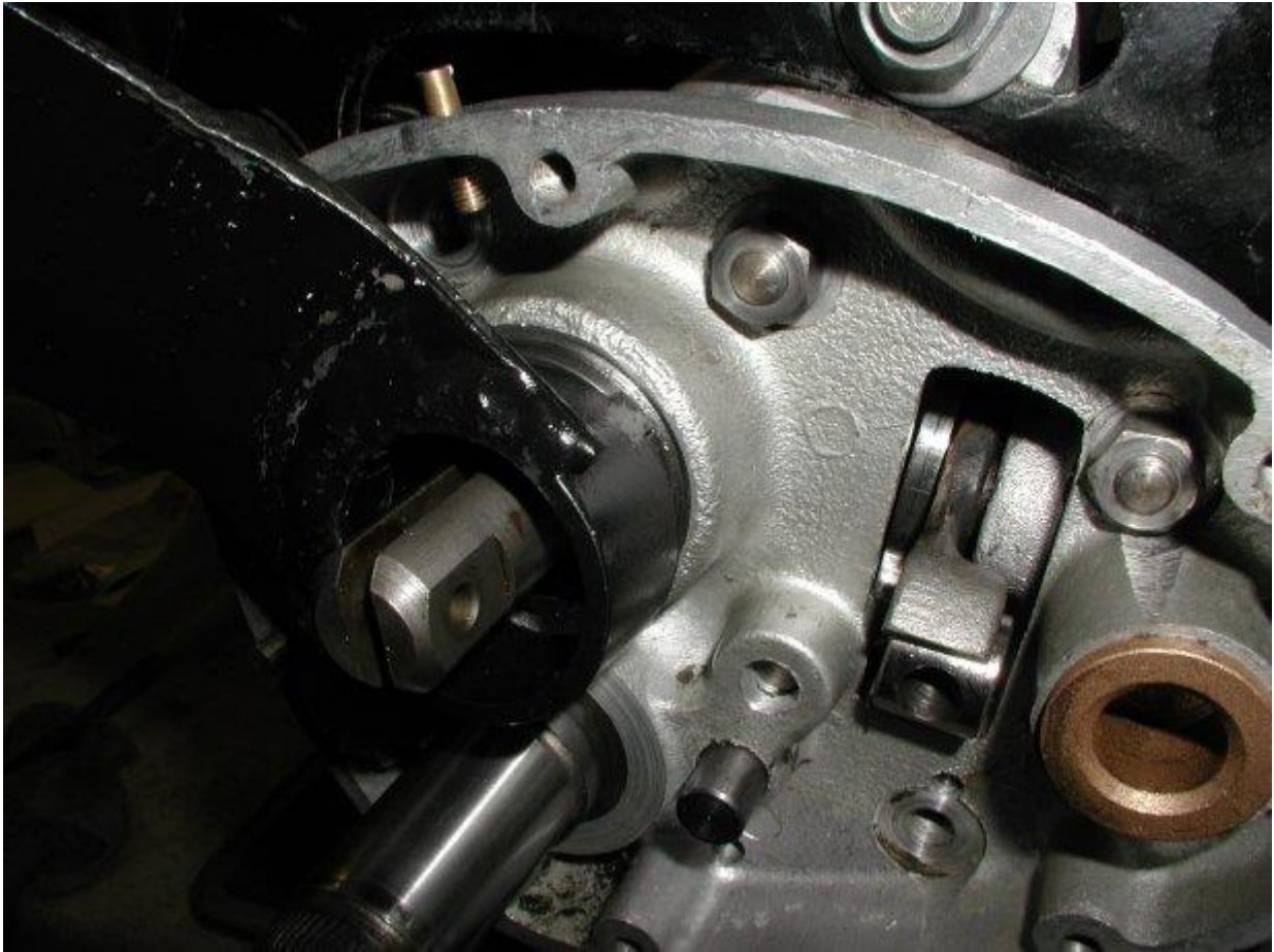
Removing the clutch operating lever body with a home built tool.
