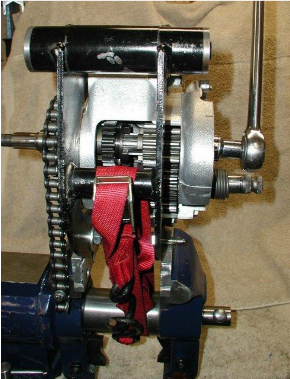
Strapping the gearbox for removing a stubborn main shaft nut.
