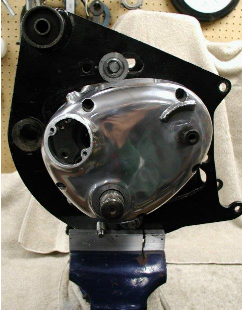
Gearbox mounted to the rear engine cradle and bolted securely in a vice.
