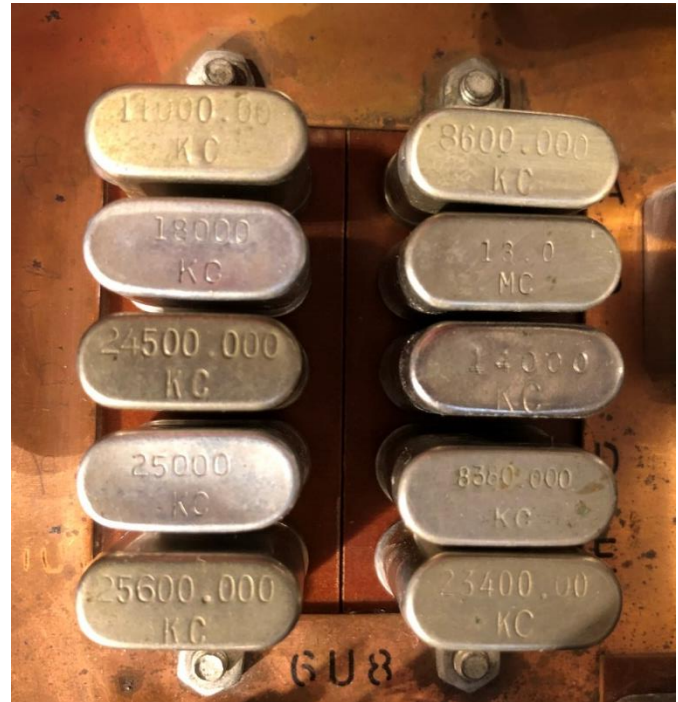
Above left: Q-Multiplier chassis after clean-up. Above right: crystal bank on the 2B chassis - the left-hand row is the standard ham band set of crystals, and the right-hand row is for 'auxiliary' frequency coverage crystals. Below: the 2B front panel after refurbishment, here receiving a station on the Broadcast Band with the 2-LF converter installed (upconverting to one of the 10M bands)
