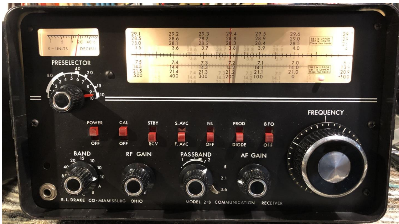
Above left: Q-Multiplier chassis after clean-up. Above right: crystal bank on the 2B chassis - the left-hand row is the standard ham band set of crystals, and the right-hand row is for 'auxiliary' frequency coverage crystals. Below: the 2B front panel after refurbishment, here receiving a station on the Broadcast Band with the 2-LF converter installed (upconverting to one of the 10M bands)
