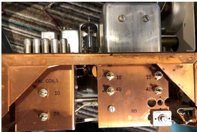
Above: underside of the Q-multiplier chassis – a simple but very effective circuit. Left: side of chassis showing the preselector adjustment slugs and trimmer. Below: rear apron showing Band E preselector adjustment slug, Q-multiplier socket, antenna and other connections. The two trimmer pots on the left hand side are for S-Meter sensitivity and 'Receiver Sensitivity' (actually AGC 'bias' or delay)
