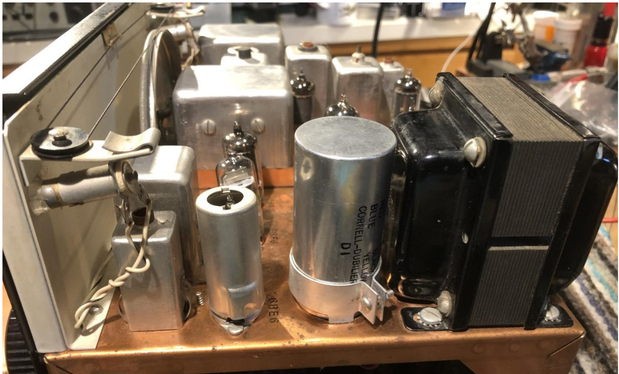
Above: chassis after cleaning and refurbishment – pity about the state of the copper plating. The crystal calibrator /2-LF socket can be seen lower-centre. Below: the replacement (re-stuffed) electrolytic can installed on the chassis – looks much like the original fitment
