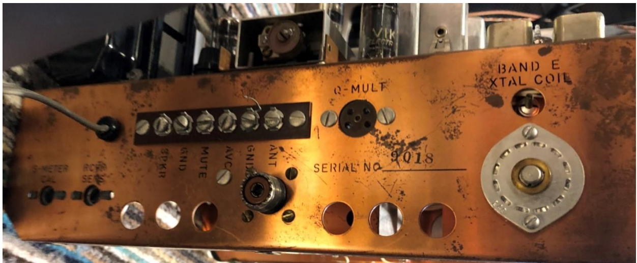
Above: underside of the Q-multiplier chassis – a simple but very effective circuit. Left: side of chassis showing the preselector adjustment slugs and trimmer. Below: rear apron showing Band E preselector adjustment slug, Q-multiplier socket, antenna and other connections. The two trimmer pots on the left hand side are for S-Meter sensitivity and 'Receiver Sensitivity' (actually AGC 'bias' or delay)
