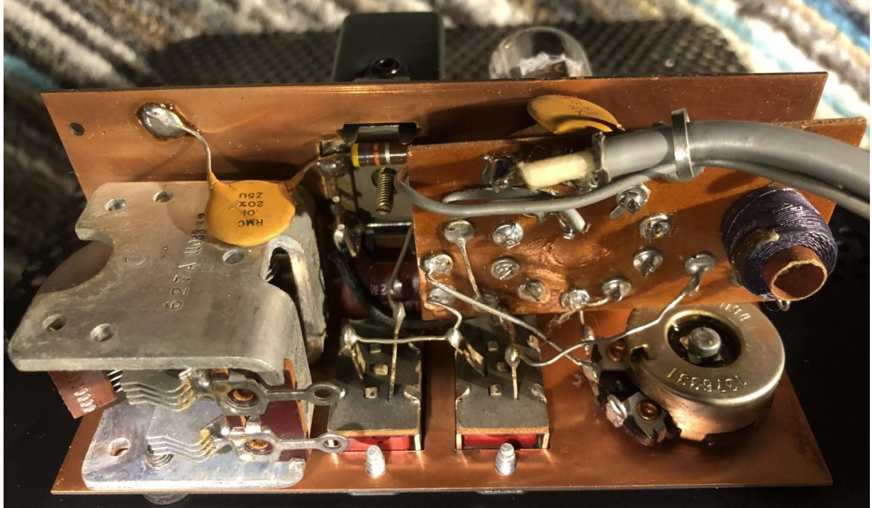
Above: underside of the Q-multiplier chassis – a simple but very effective circuit. Left: side of chassis showing the preselector adjustment slugs and trimmer. Below: rear apron showing Band E preselector adjustment slug, Q-multiplier socket, antenna and other connections. The two trimmer pots on the left hand side are for S-Meter sensitivity and 'Receiver Sensitivity' (actually AGC 'bias' or delay)
