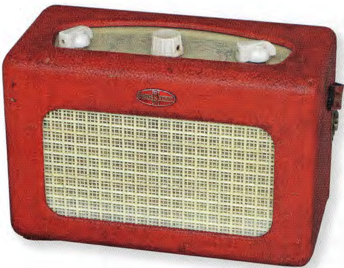
Shown above is the radio seated in its upright "playing" position. The speaker is located behind the grille, as shown in the photo to the right. The radio can run from either 200-250VAC mains or two dry batteries, one rated at 90V for HT and the other at 1.5V for LT.
