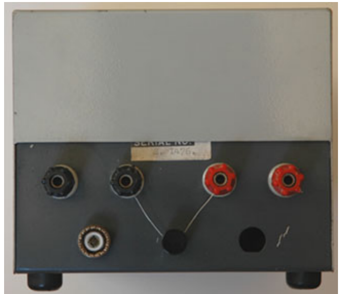
Photo #2 Antenna connections at the rear of the unit are two pairs of terminals each capable of accepting banana-plugs, spade-tag or simply screw down on to a wire.
