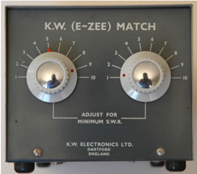
Photo #1 Front panel controls. Left knob is the Shunt capacitor adjustment and the Right knob is the Source Load capacitor adjustment.
